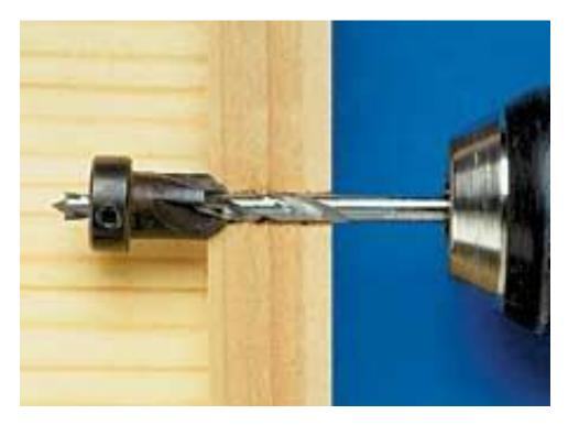
First reverse the countersink cutter on the end of the drill bit, as shown in the photo. Then insert the bit through the pilot hole and chuck it in the drill. Now to countersink the hole, all you have to do is reverse the direction of the drill and gently pull back on the bit.
