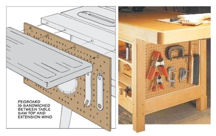
To add storage to your workbench, you can nail some cleats to the legs and upper and lower end rails of the bench (above right). Then place the pegboard against the cleats and tack a second set of cleats down to hold the pegboard in place.
