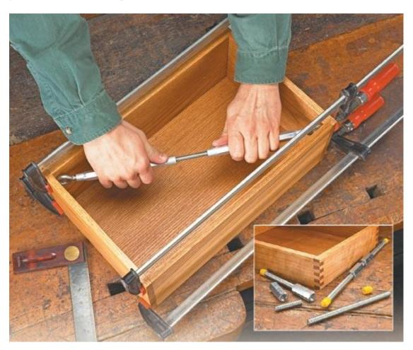
The concept is pretty simple. The squaring rods are used to apply pressure across the short diagonal of the drawer to push it into square. For large drawers I have a squaring rod consisting of a section of threaded rod, two turnbuckles and a couple of eyebolts. As you can see, the eyebolts wedge into the corners of the drawer to force it into square.
