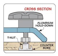
To make this modification, just drill a  $^5/_{16}$ " hole at one end of the sled that will accept a short piece of threaded rod. The location of the hole depends on the type of hold-down you'll be using. It just needs to be located close enough for the hold-down to secure a small workpiece firmly in place.
