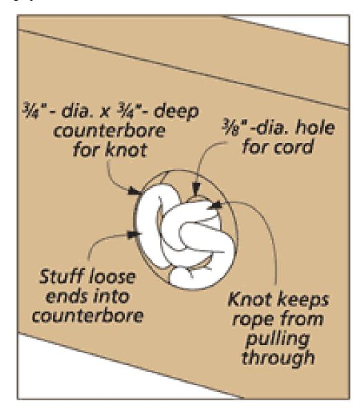
The wall rack consists of a board outfitted with a series of "hook and loop" cord holders. The loops are made from 1' long sections of nylon cord. The cord is knotted in a loop and then passed through a counterbored hole in the board, as shown in the drawing. An eye hook installed above the cord completes the holder.
