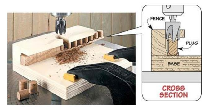
The jig, shown in the photo above, is made up of two parts. The first part is a small (6" x 12") plywood base that gets clamped to the drill press table for stability. The second part is a hardwood fence that prevents lifting of the workpiece and guides the plug stock and the plug cutter.
