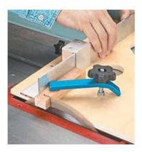
One of the problems using a cut-off sled is that as the workpieces get shorter, your fingers get closer and closer to the blade. To solve this problem, I simply added a hold-down to the sled, like the one you see in the photograph at right.
