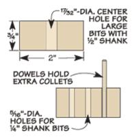
The system consists of 2"-square MDF "tiles" that hold the bits. The tiles keep the cutting edges from hitting each other. For largediameter bits, I drilled a single, centered shank hole. For smaller bits, you can drill several holes in one tile. I even mounted a pair of dowels in one tile to hold extra collets. The individual tiles make it easy to rearrange and expand the system as you add new bits.
