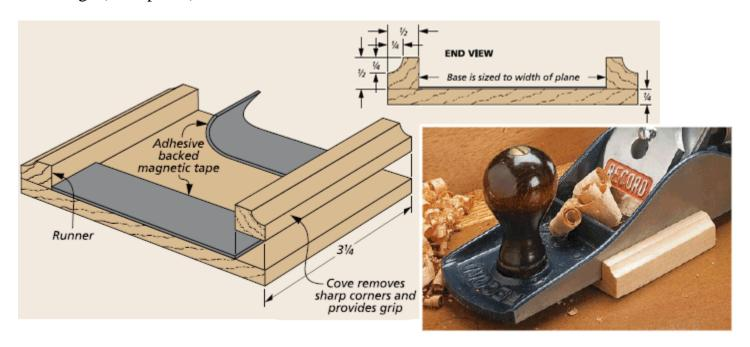
As you can see in the drawings, the saddle is very simple. A thin hardwood base, sized to fit the plane, serves as a platform. A runner on either side of the base creates a channel for the plane. To prevent the plane iron from contacting the base, I added a strip of soft, adhesive-backed magnetic tape to each end. The tape also serves to hold the saddle in place.
