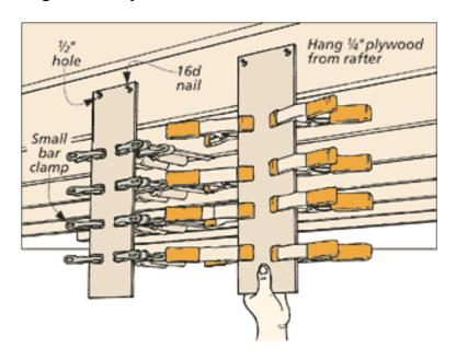
As you can see in the drawing at right, my small clamp storage merely consists of a couple pieces of ½" plywood hanging from the joists of my basement shop. Each piece of plywood simply slips over a couple of large nails. When I need a clamp or two, I simply reach up, lift the plywood off its hangers and remove the clamps I need.
