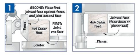
Now you're ready to move to the planer. Place one of the jointed faces down on the planer bed, and make a pass. Then flip the piece 90° again to plane the adjoining face. Continue making passes through the planer this way until the pieces reach the desired width and thickness (*Fig. 2*).
