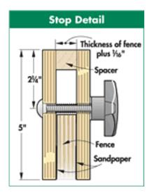
Tightening a knob on a carriage bolt that passes through both pieces of plywood clamps the stop block to the fence. A strip of sandpaper (for a wood fence) or rubber (for a metal fence) attached to the inside faces of the stop block provides a firm grip on the fence.
