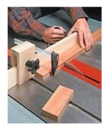
Stop blocks are an indispensable accessory when cutting pieces to length on the table saw or miter saw. And they don't get much simpler or quicker to make than this one.
