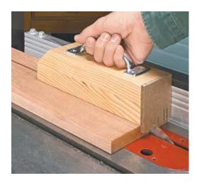
I find many push sticks somewhat unnerving to use. So I made a sturdy push block for my table saw that keeps my hand well above the blade. And the wide body of the block pushes the workpiece on both sides of the saw blade.
