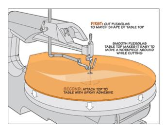
Most of the work I do on my scroll saw involves fine cuts on small pieces. So it's very important for the workpiece to slide easily across the table. The problem is most scroll saw tables aren't very smooth. I've tried waxing the table and found that the wax wears off pretty quickly and leaves a residue on my projects.
