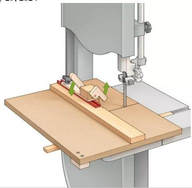
For the sled base, I used 3/4" MDF. On the underside, I attached a runner to slide in the saw's miter slot. I also attached a small stop block under one corner of the base to prevent the fence from sliding too far into the blade.
