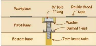
With this jig you can accurately and repeatably cut circles of various diameters, even when months pass between work sessions. Simply mark and drill 7mm or  $\frac{9}{32}$  "holes at various radii in the bottom base. Then, insert short lengths of 7mm brass tube, the kind sold for making slim pens, and secure them with cyanoacrylate (instant) glue. Install a  $\frac{1}{4}$  "bolt into the pivot base. The bolt fits snugly in the 7mm tube.
