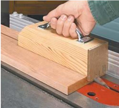
I find many push sticks somewhat unnerving to use. So I made a sturdy push block for my table saw that keeps my hand well above the blade. And the wide body of the block pushes the workpiece on both sides of the saw blade.
